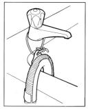
2. In all cases, check that the end of the drain hose is securely fixed to prevent the repulsive force of the water from pushing it out of place.
